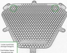
Push Rubber Spacer through from the back of the guard so Hexagonal shape sits on the front face
